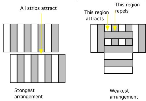
b) The vibration occurs when the magnets are slid apart while the strips are held parallel. During a fraction of a second the magnets are attracted to each other, a split second later, they are repelled. This jerking motion feels like your magnets are vibrating.
